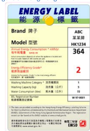
Figure 9: Hong Kong China VEELS Energy Label for a Washing Machine. The label shows an Energy Efficiency Grade of 2 (yellow), indicating it is 'Average'. Key specifications include: Brand (ABC), Model (HK1234), Annual Energy Consumption (kWh/year) of 364, Washing Machine Category (1), Washing Capacity (kg) of 5, Water Consumption (liters) of 72, and an EEL Registration Number (W 97-0001). The label is issued by the Electrical and Mechanical Services Department (EMSD).
