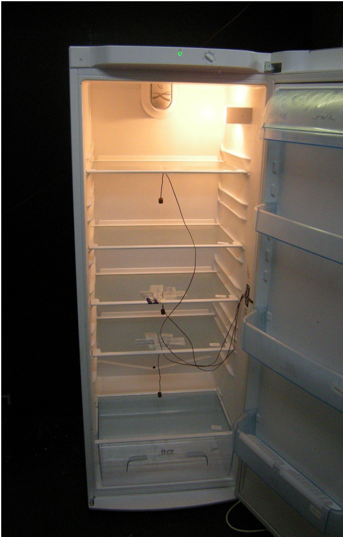
Figure 1 & 2 – Photo showing fridge under test with thermocouples in place.
