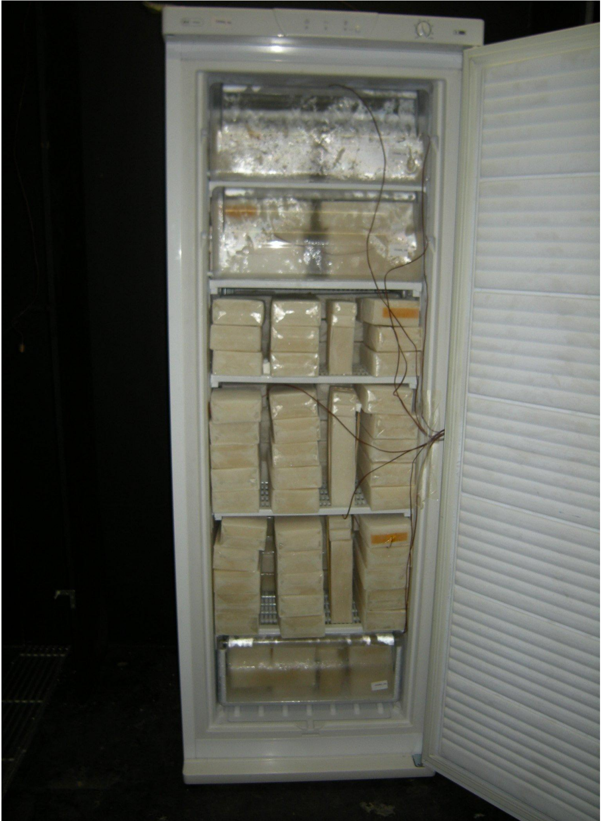
Figure 2 - Photo of a freezer loaded with test packages and thermocouples in place.
